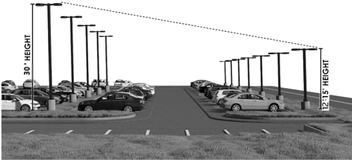
Figure 6.6.2 Parking Area Lighting Standards Illustrative Example
