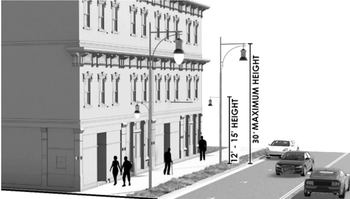
Figure 6.6.1. Lighting Fixture Height Illustrative Example
