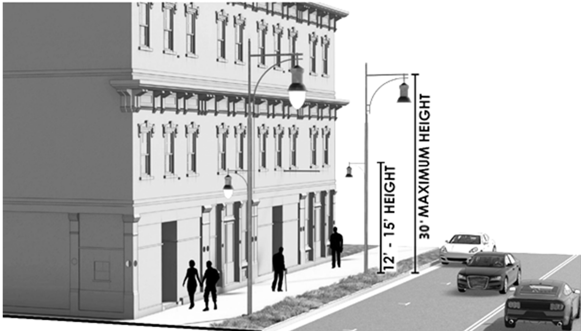
Figure 6.6.1. Lighting Fixture Height Illustrative Example
