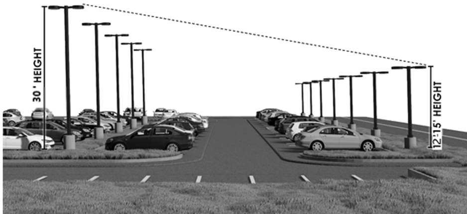
Figure 6.6.2 Parking Area Lighting Standards Illustrative Example
