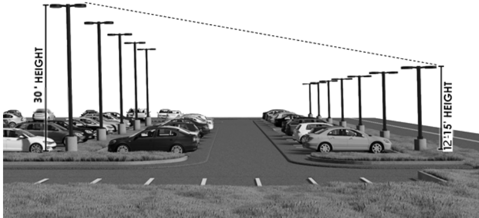
Figure 6.6.2 Parking Area Lighting Standards Illustrative Example
