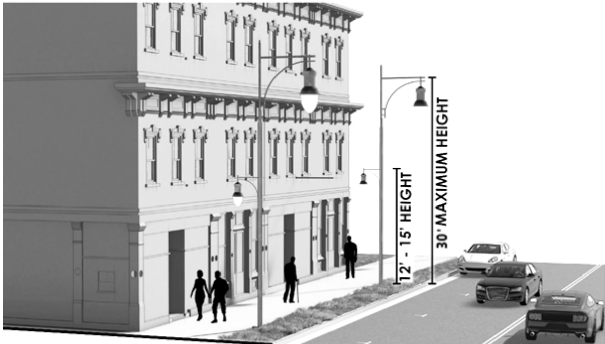
Figure 6.6.1. Lighting Fixture Height Illustrative Example
