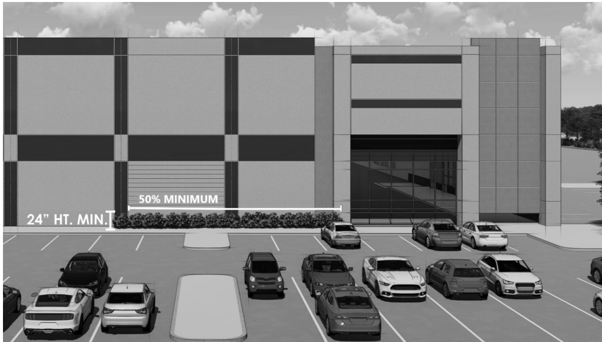
Figure 6.8.9. Industrial Use Foundation Plantings
