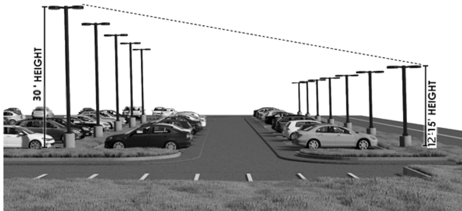
Figure 6.6.2 Parking Area Lighting Standards Illustrative Example
