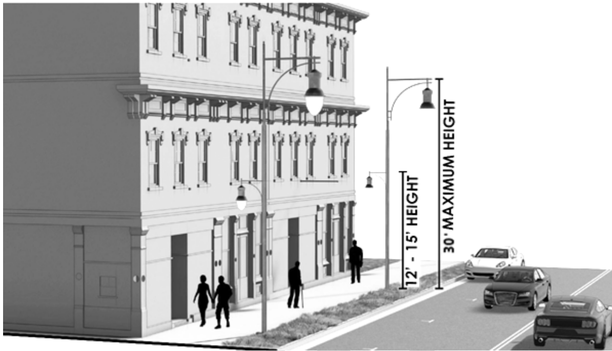
Figure 6.6.1. Lighting Fixture Height Illustrative Example
