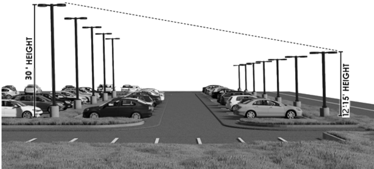
Figure 6.6.2 Parking Area Lighting Standards Illustrative Example
