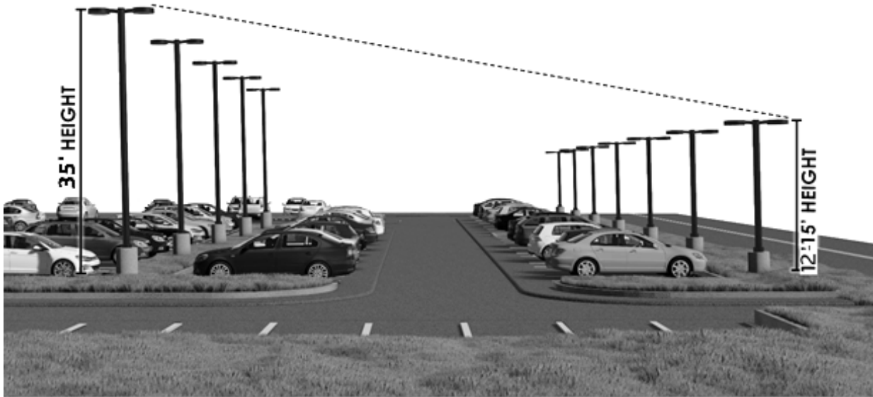
Figure 6.6.2 Parking Area Lighting Requirements
