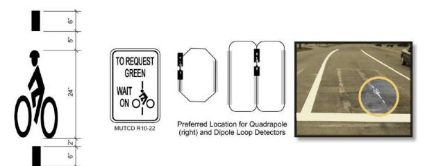
Figure 4-6. Bicycle Position Stencil for Signal Loop Detector
