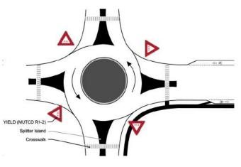
Figure 1-7. Modern Roundabout Design
