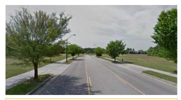
Redford Place Drive is at the upper limit of a typical low-volume collector or residential street. The particular design and infrequent curb cuts of this road might suggest dedicated bicycle lanes; such a prescription would probably preclude a center turn lane due to the costs of relocating utilities, curbing and landscaping that would be necessary were the center turn lane retained. Sharrows markings would be a good intermediate step.
