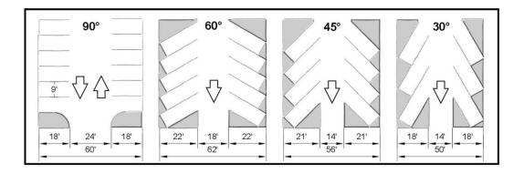
\* If angle degree parking bay is design in opposite angle direction on either side the travel lane the width will be 24 ft. The Travel Lane + Parking Bay width will include the increase travel lane width.
