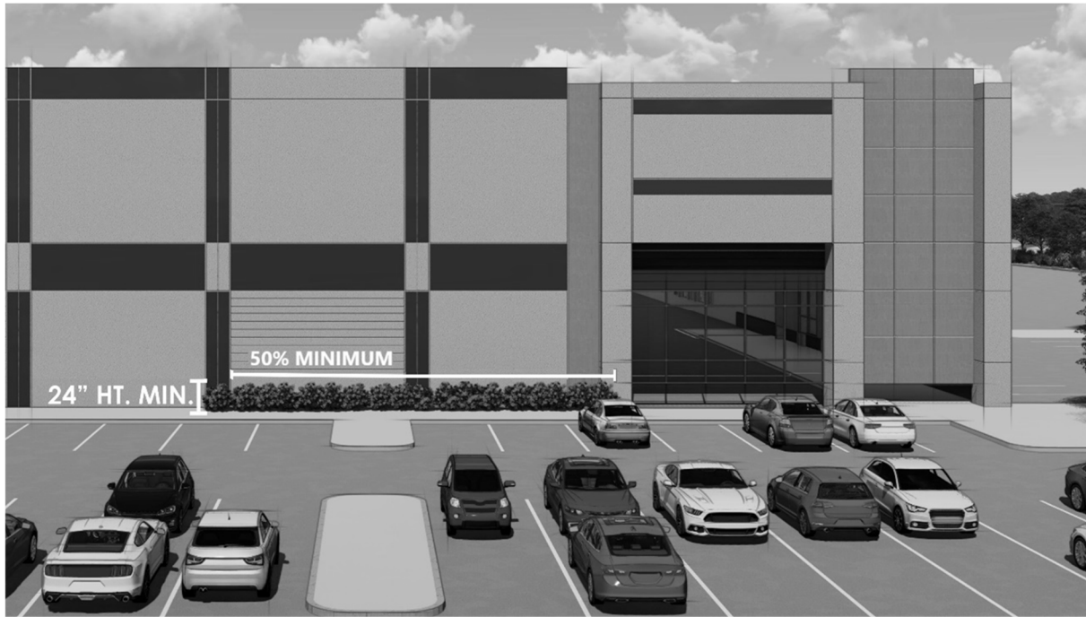
Figure 6.8.9. Industrial Use Foundation Plantings
