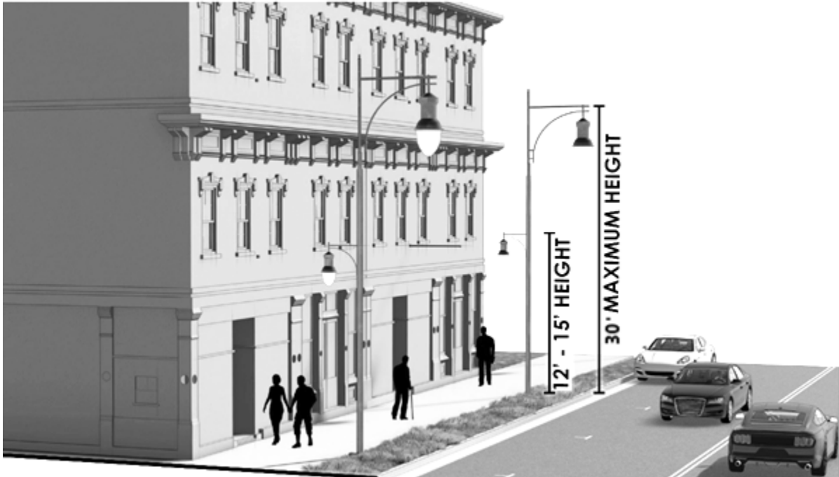
Figure 6.6.1. Lighting Fixture Height Illustrative Example
