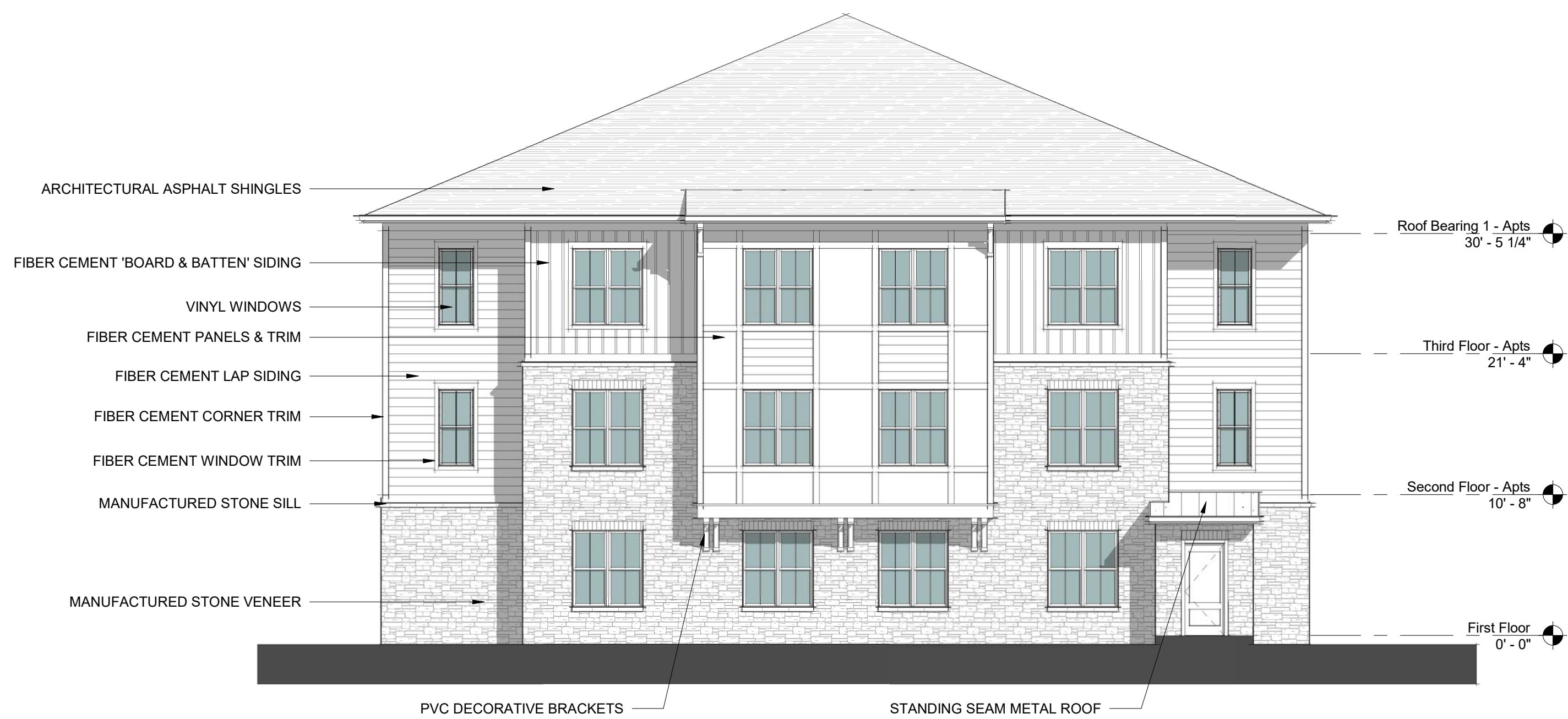
BLDG 8 - LEFT SIDE ELEVATION 3 1/8" = 1'-0"
