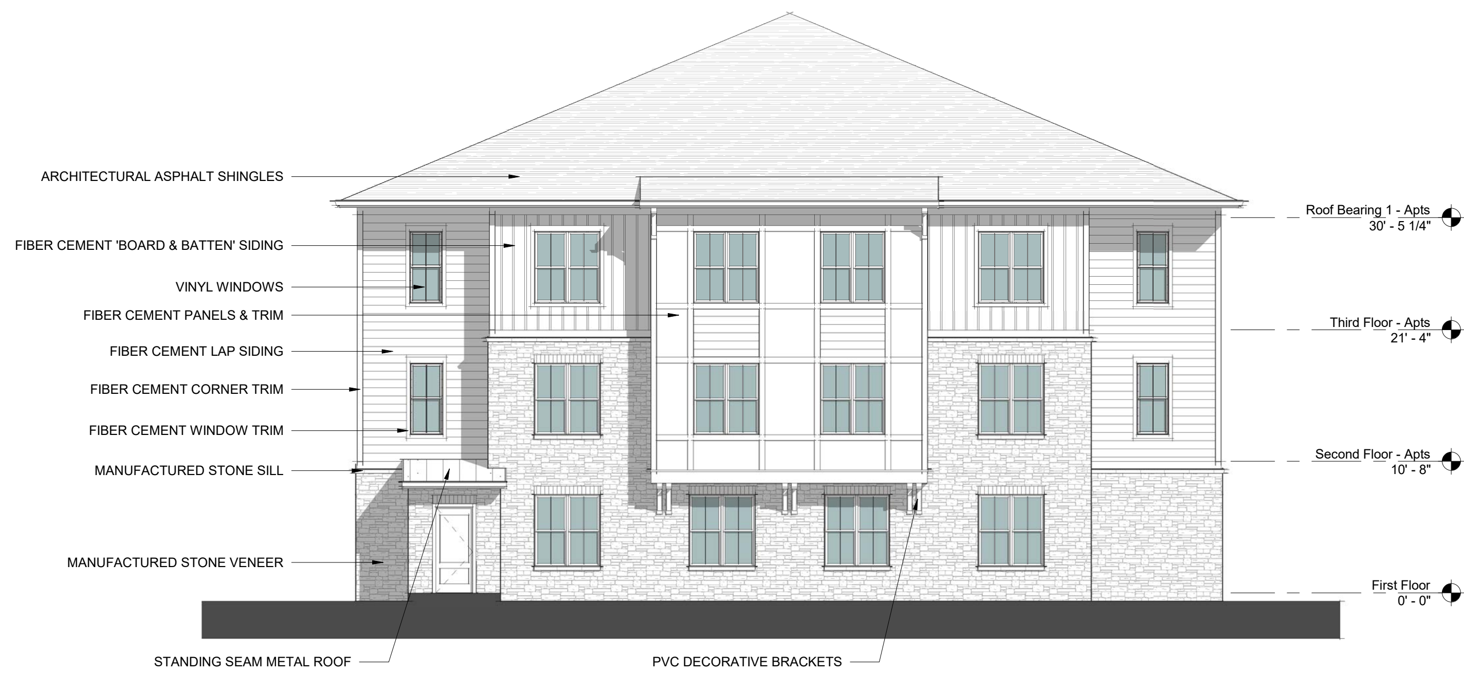
BLDG 8 - RIGHT SIDE ELEVATION 4 1/8" = 1'-0"
