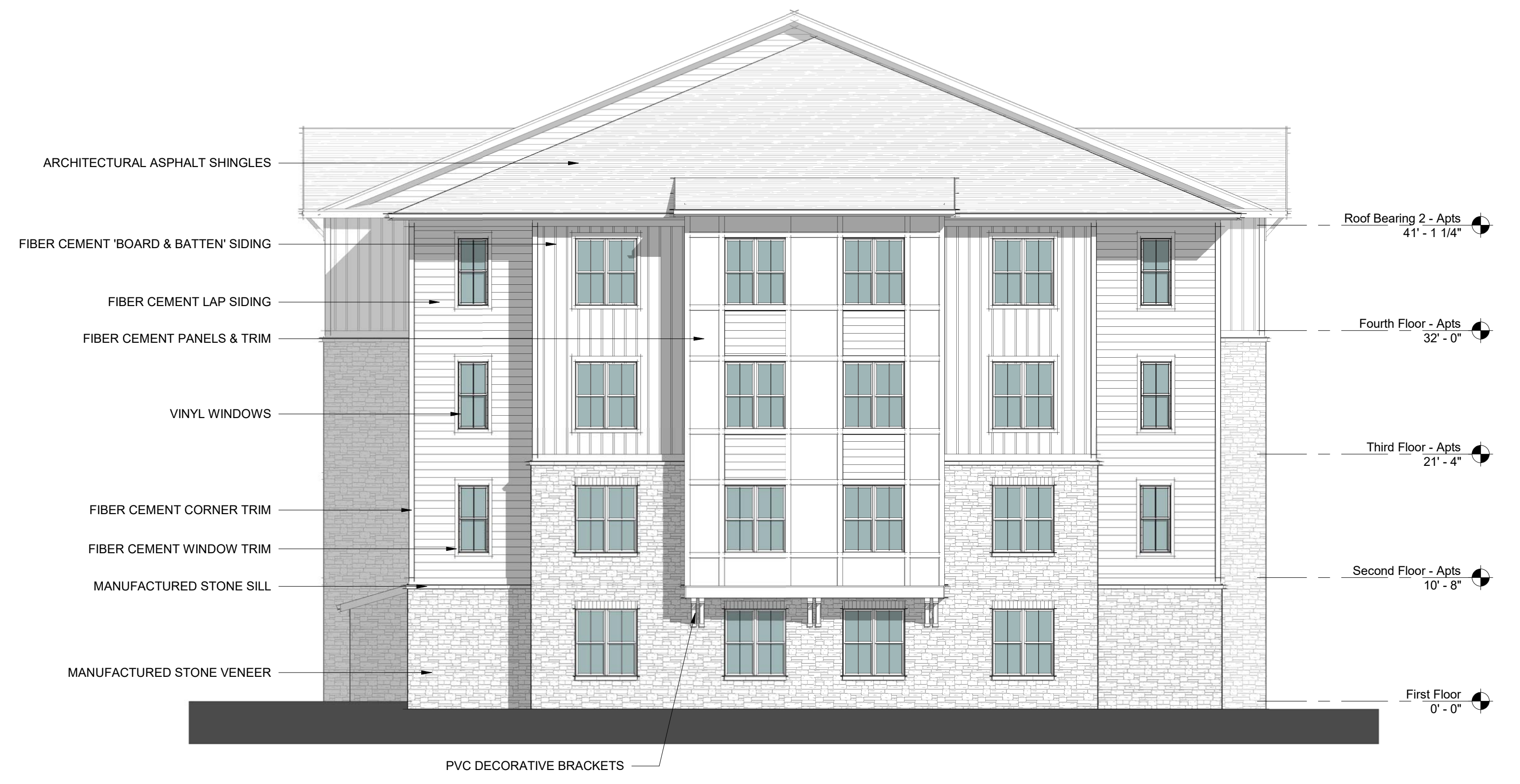
BLDG 1 & 7 - RIGHT SIDE ELEVATION 1 1/8" = 1'-0"
