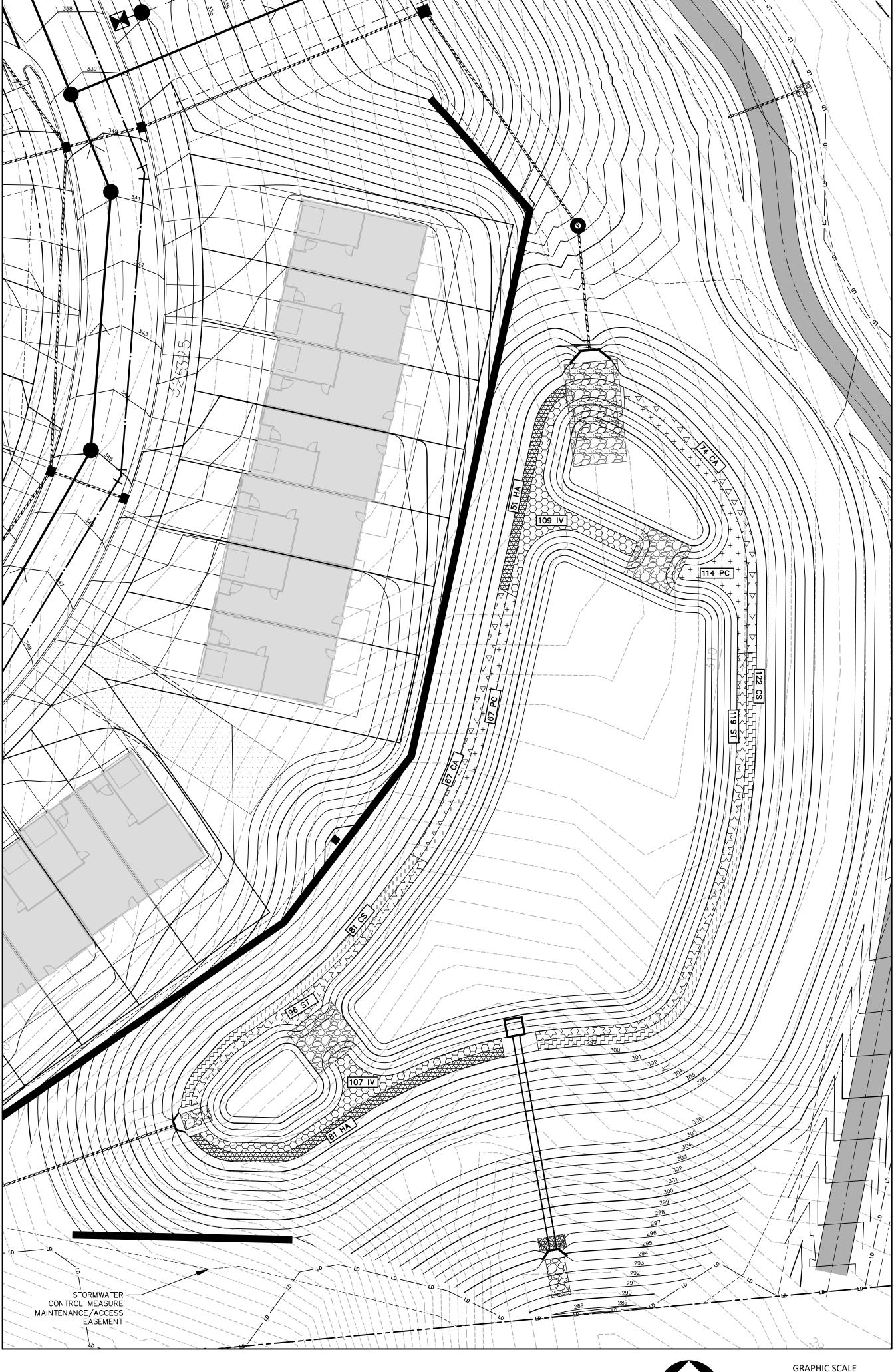
STORMWATER CONTROL MEASURE 'K' PLAN VIEW
