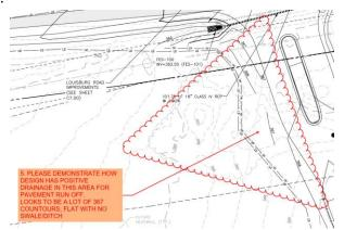
McAdams Response: Contours have been adjusted to show positive drainage toward roadside swale and graded depression at future field swale.
