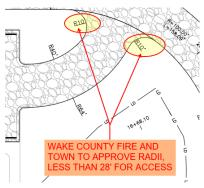
McAdams Response: Radii have been adjusted in direction of travel for fire truck access. Future modifications may be required at time of full buildout.
