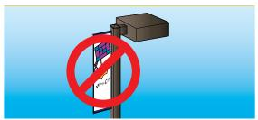
Hanging signs, banners and flags on light poles change the EPA rating and increase vibration. The EPA ratings data provided on this guide does not allow for this added stress, which could result in pole or fixture failure.
