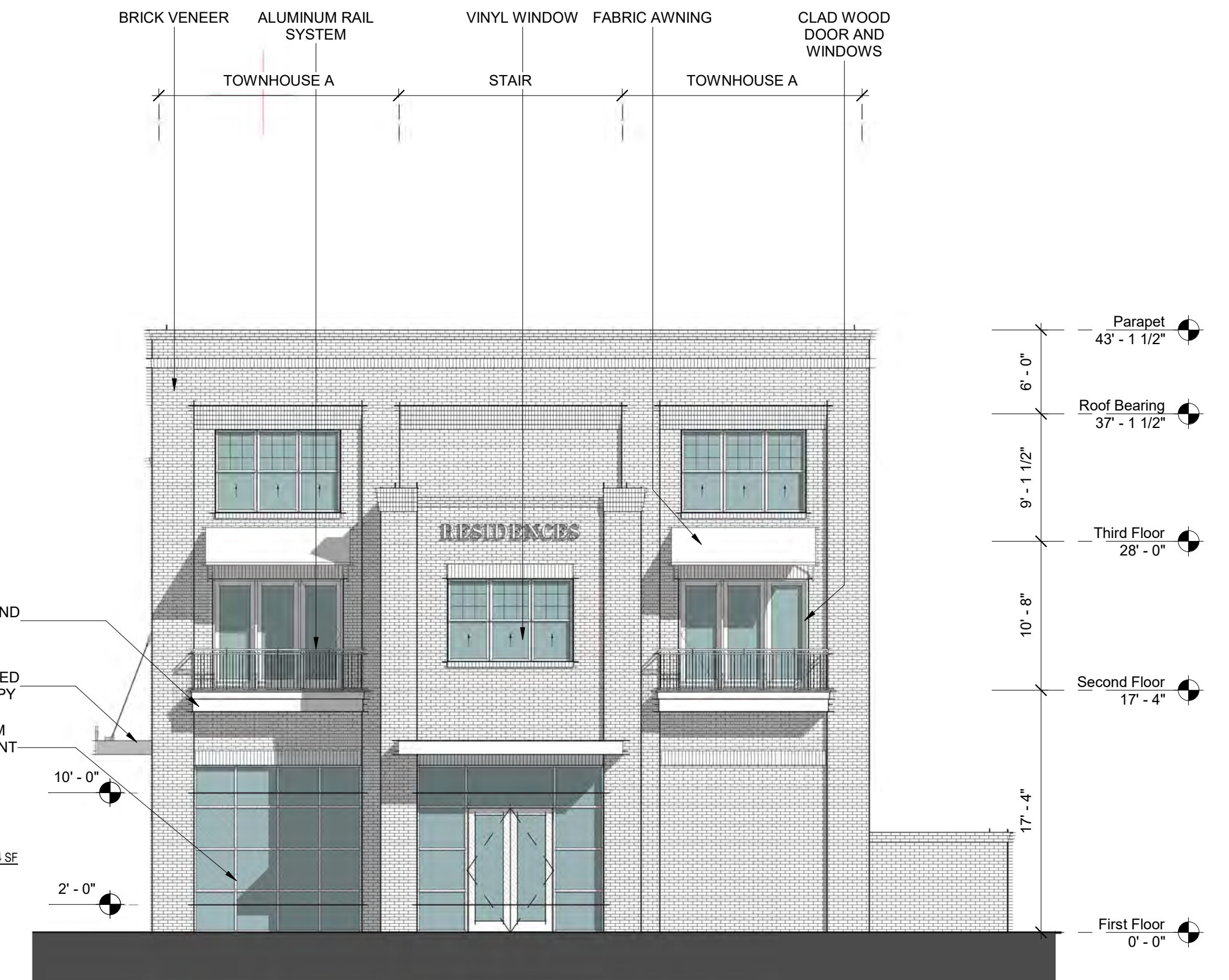
BLDG 5 - SOUTH ELEVATION 2 1/8" = 1'-0"
