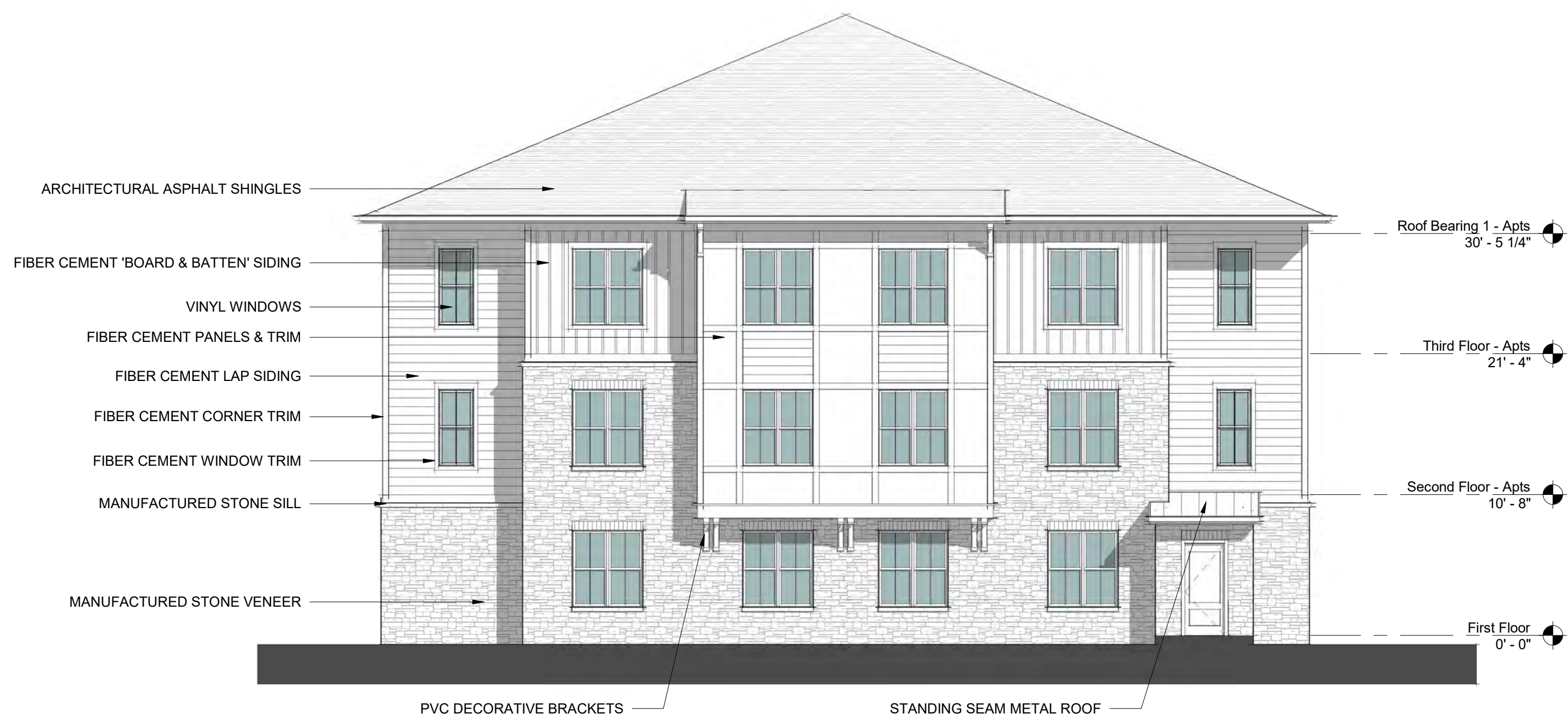
BLDG 8 - LEFT SIDE ELEVATION 3 1/8" = 1'-0"
