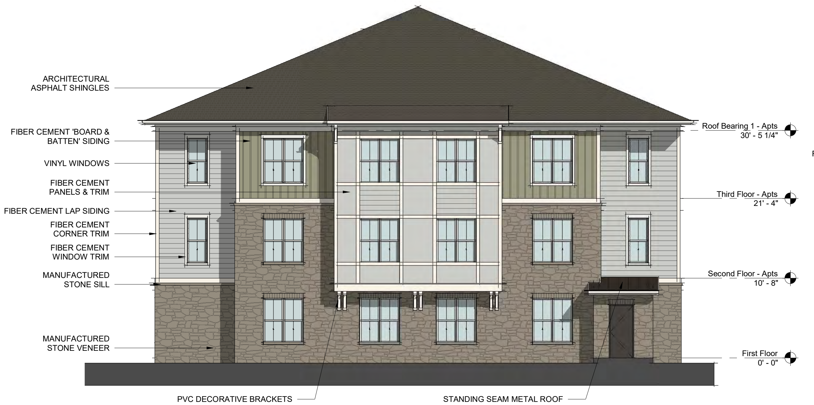
BLDG 8 - LEFT SIDE ELEVATION 3 1/8" = 1'-0"
