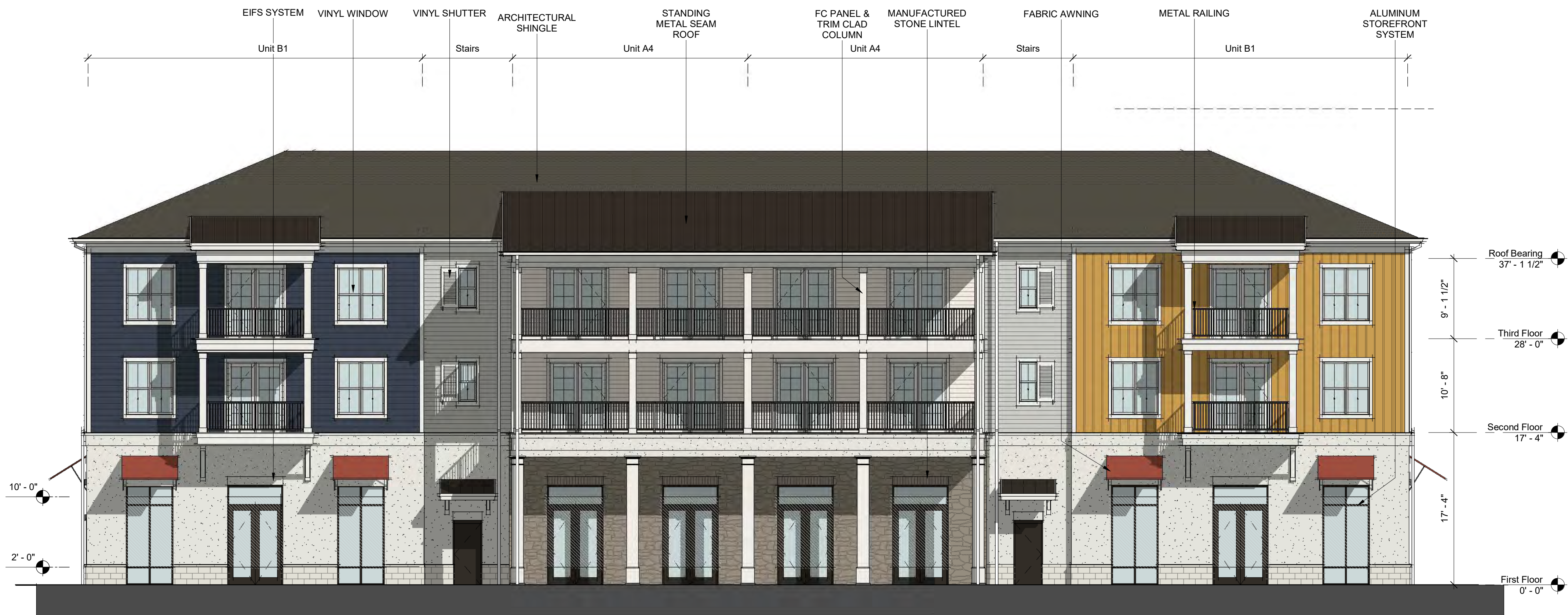
BLDG 3 - SOUTH ELEVATION 2 1/8" = 1'-0"
