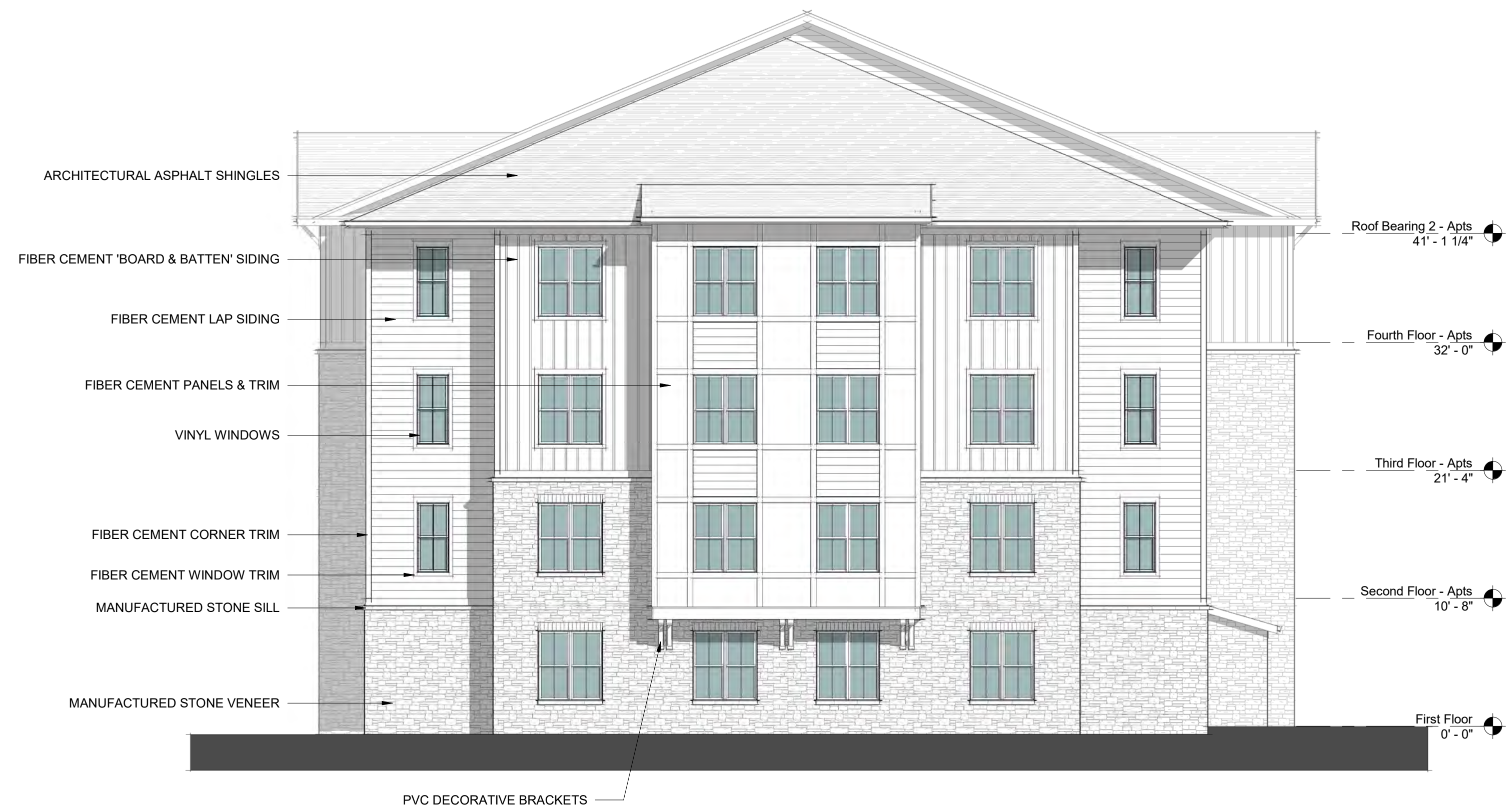
BLDG 1 & 7 - LEFT SIDE ELEVATION 2 1/8" = 1'-0"
