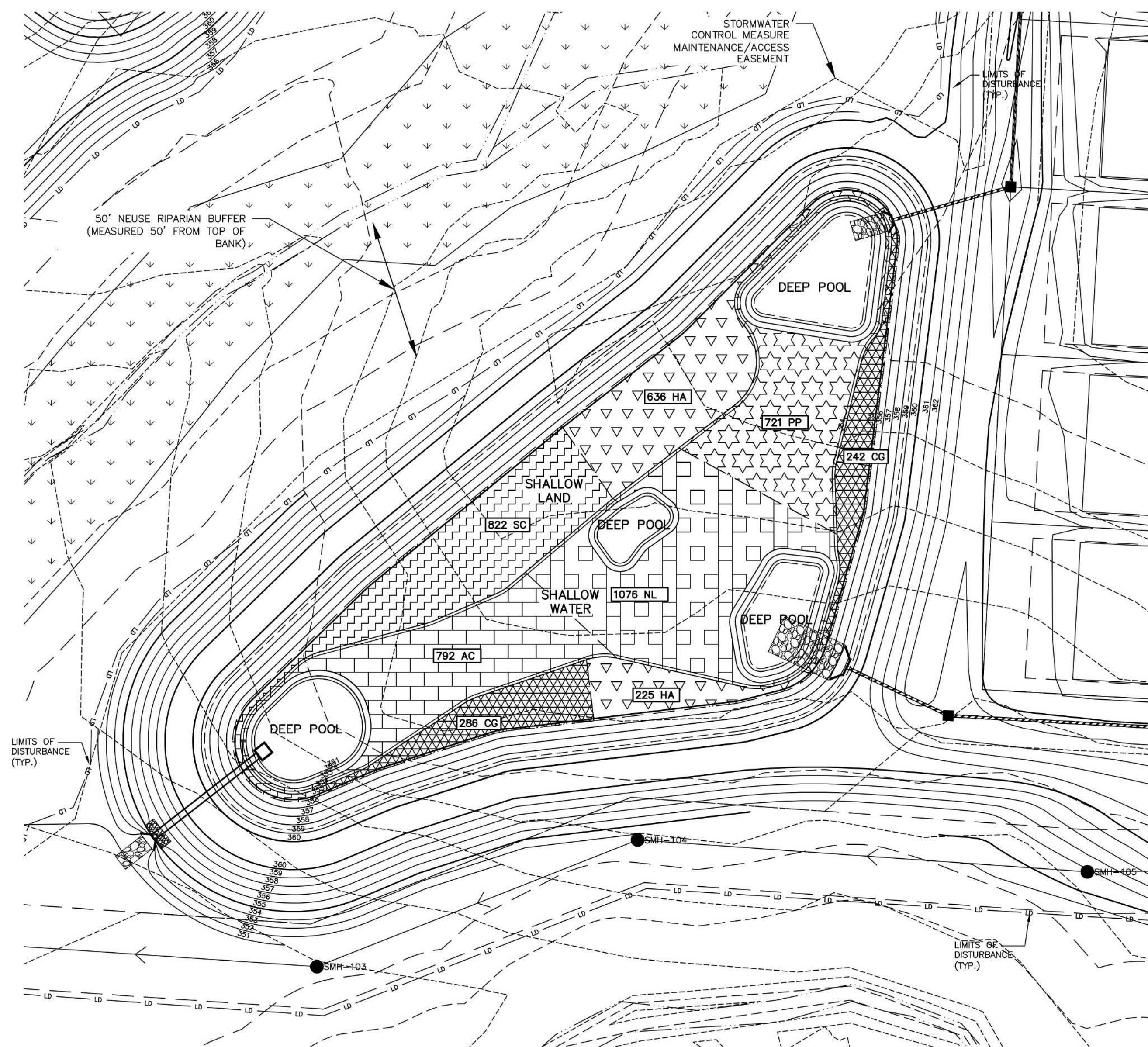
STORMWATER CONTROL MEASURE 'D' LANDSCAPE PLAN
