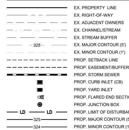
EX. PROPERTY LINE EX. MAJOR CONTOUR (5') PROP. CURB INLET (CB) PROP. YARD INLET PROP. FLARED END SECTION PROP. JUNCTION BOX PROP. LIMIT OF DISTURBANCE PROP. MAJOR CONTOUR (5') —— PROP. MINOR CONTOUR (1')
