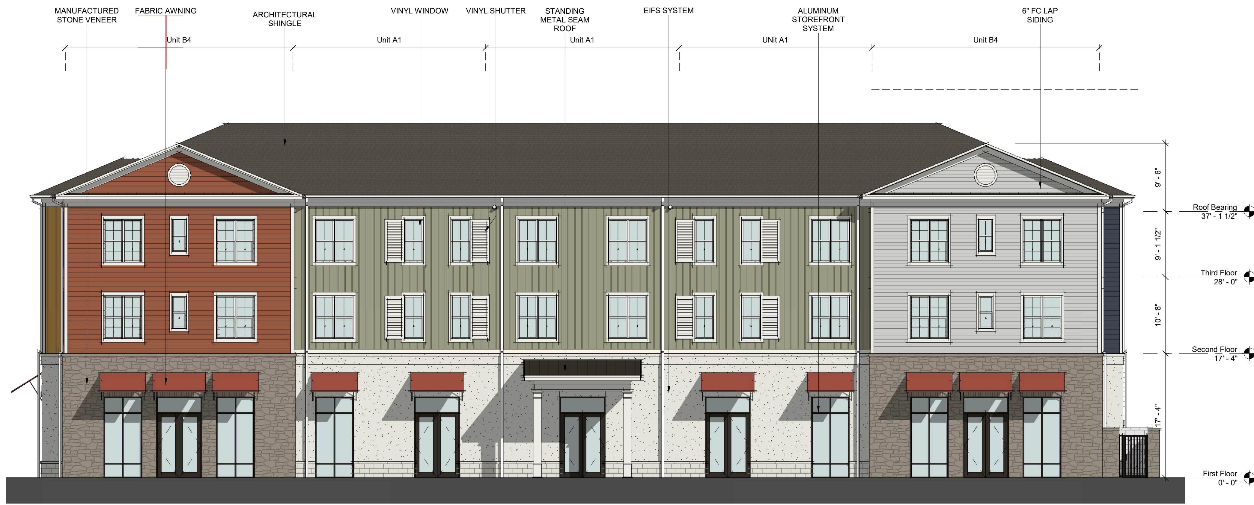
BLDG 3 - NORTH ELEVATION 1 1/8" = 1'-0"
