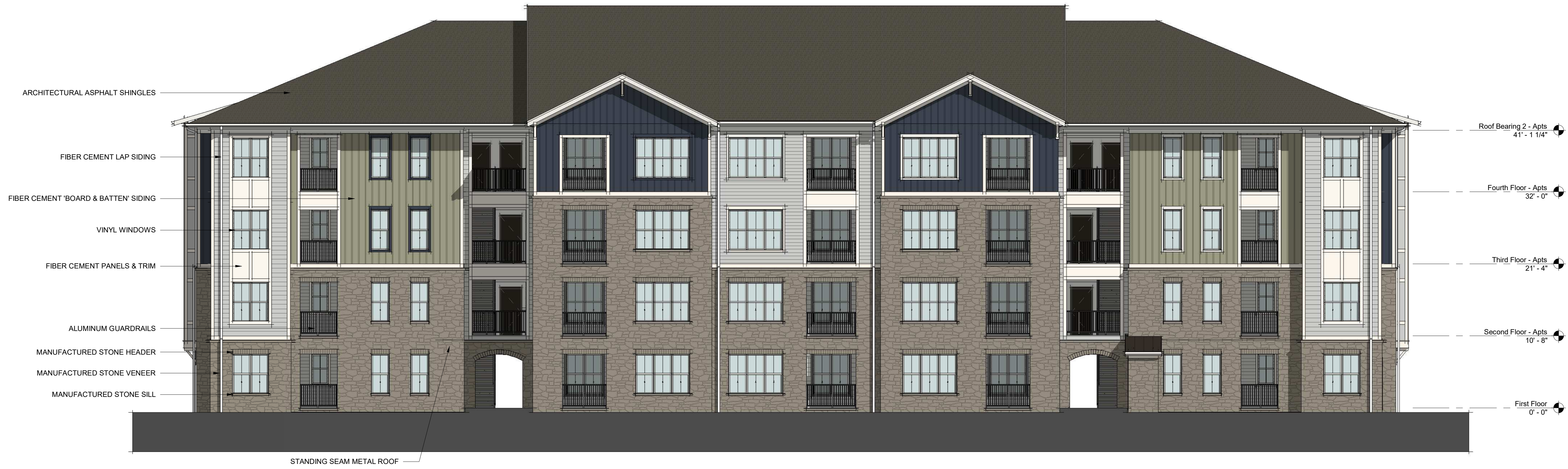
BLDG 1 & 7 - FRONT ELEVATION 1 1/8" = 1'-0"
