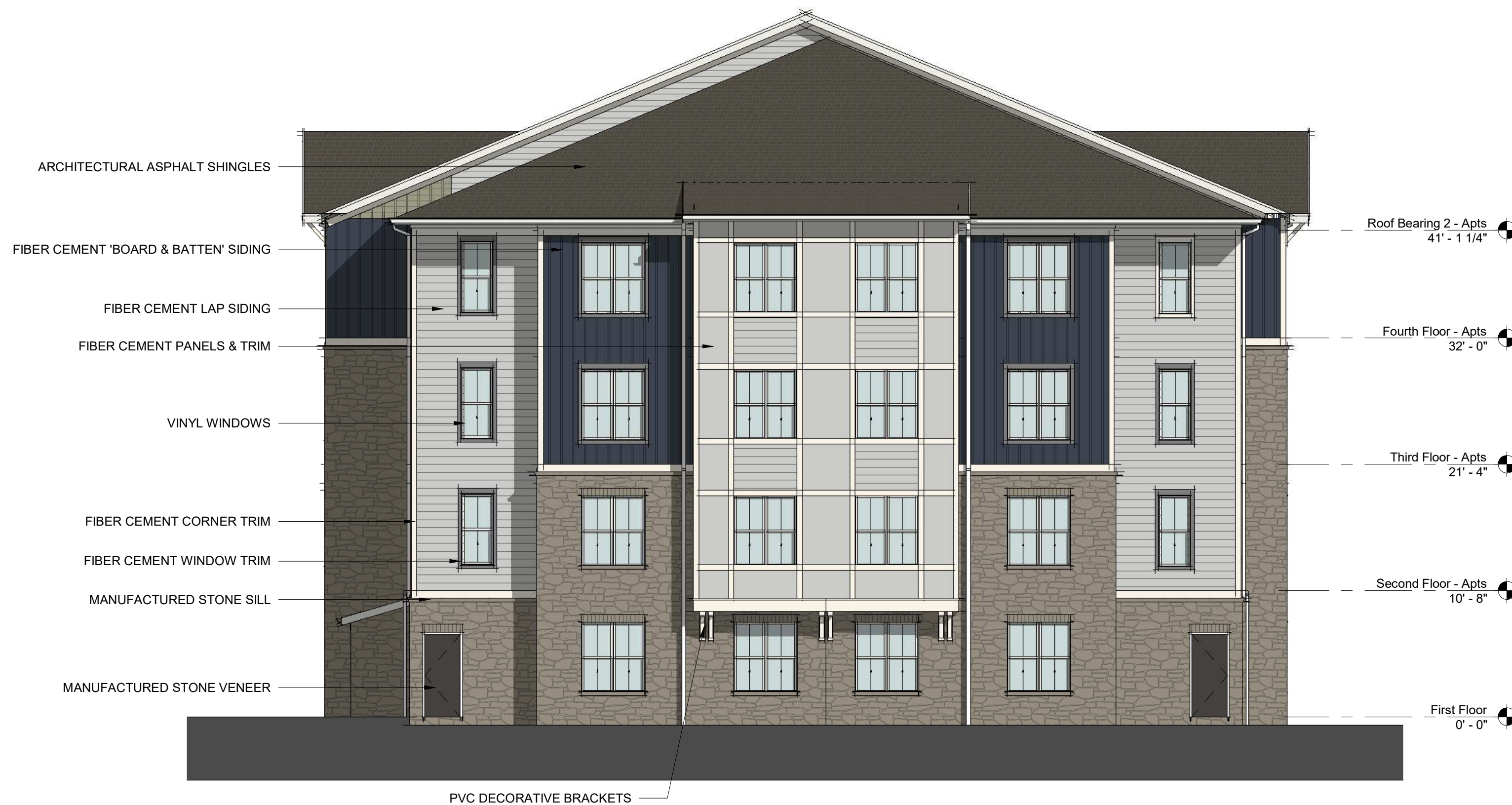
BLDG 1 & 7 - RIGHT SIDE ELEVATION 1 1/8" = 1'-0"
