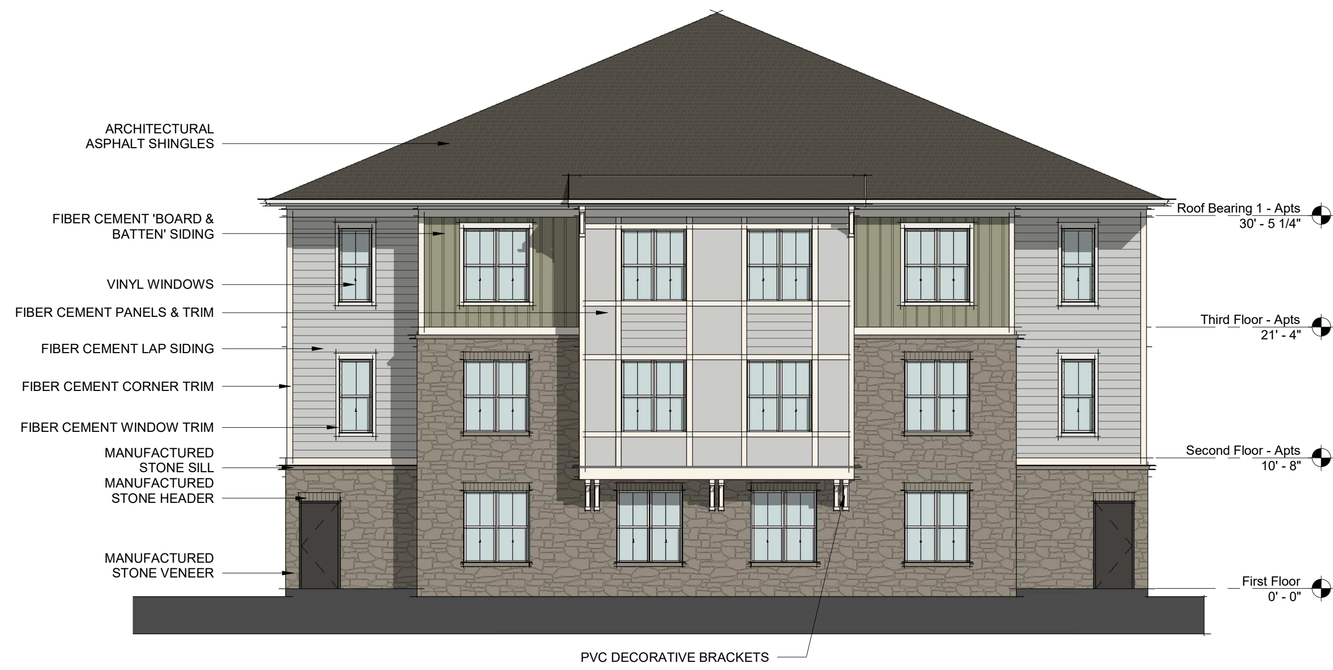
BLDG 8 - RIGHT SIDE ELEVATION 4 1/8" = 1'-0"
