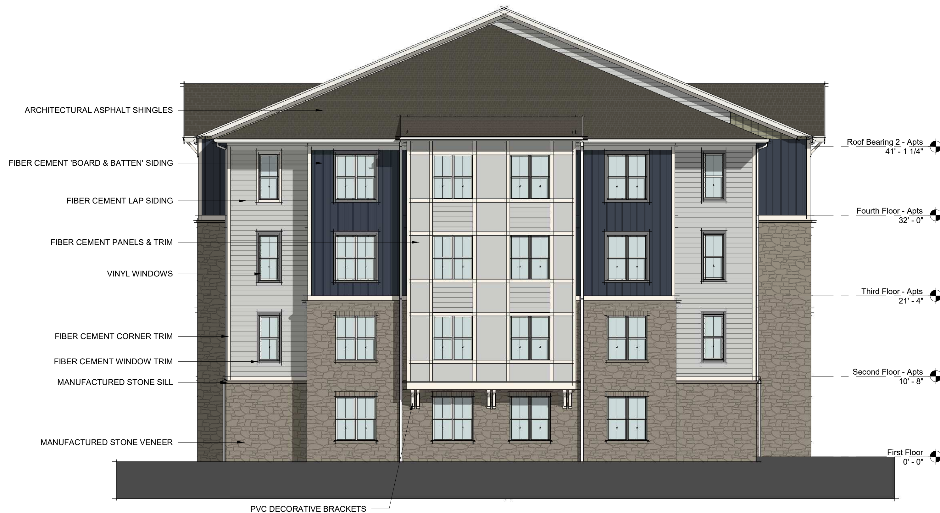
BLDG 1 & 7 - LEFT SIDE ELEVATION 2 1/8" = 1'-0"
