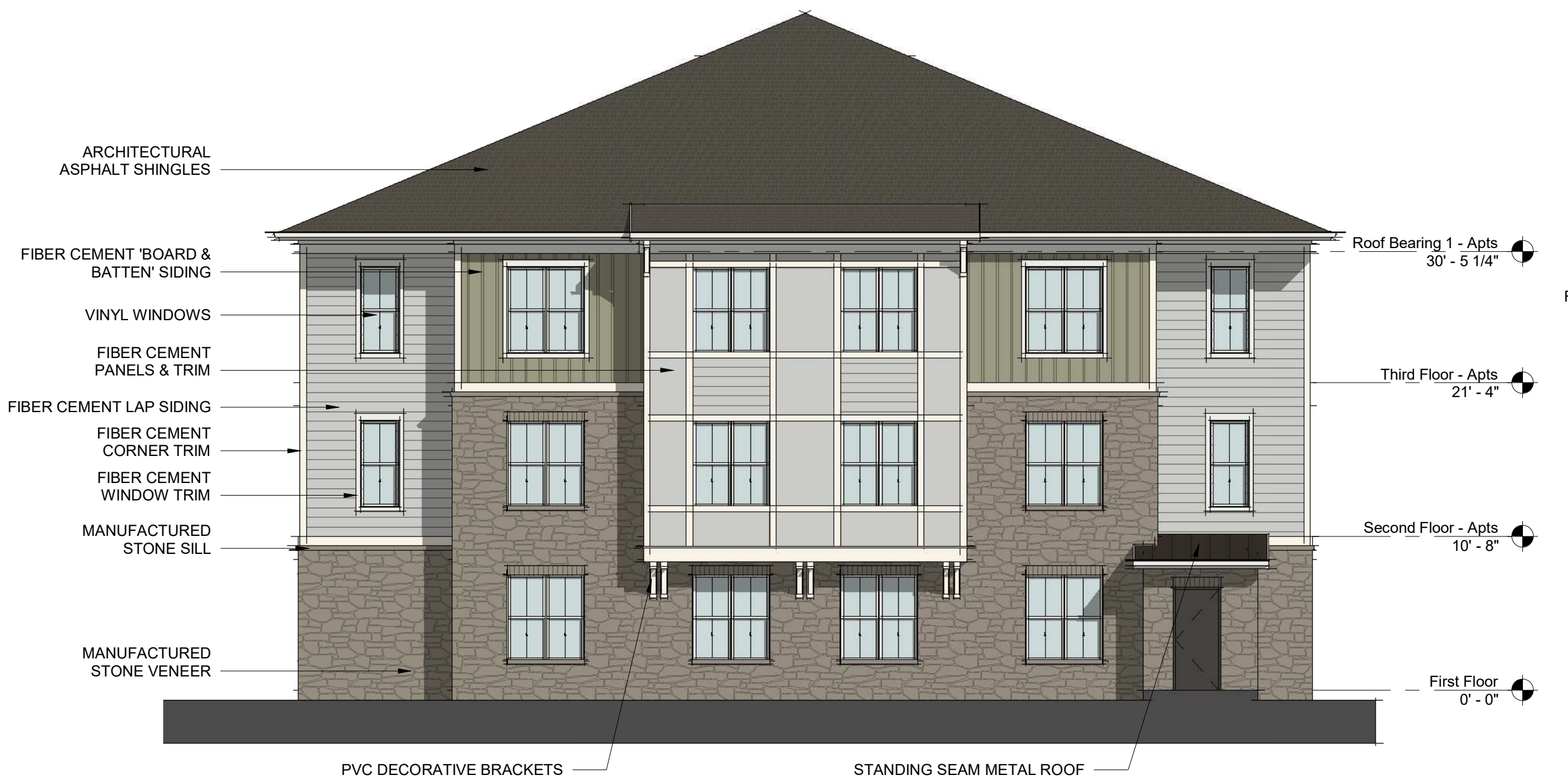
BLDG 8 - LEFT SIDE ELEVATION 3 1/8" = 1'-0"
