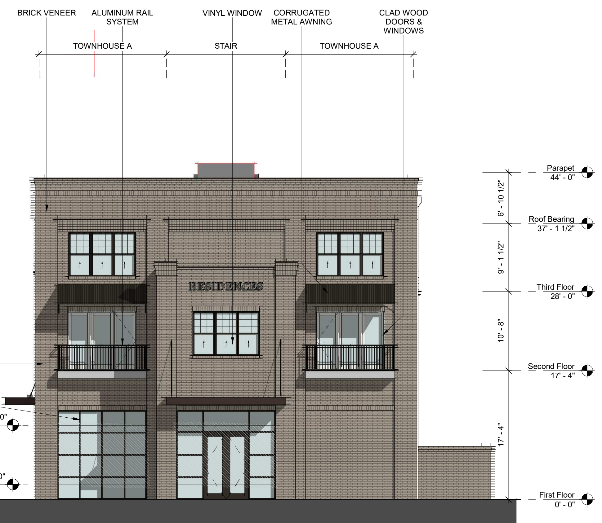
BLDG 5 - SOUTH ELEVATION 2 1/8" = 1'-0"
