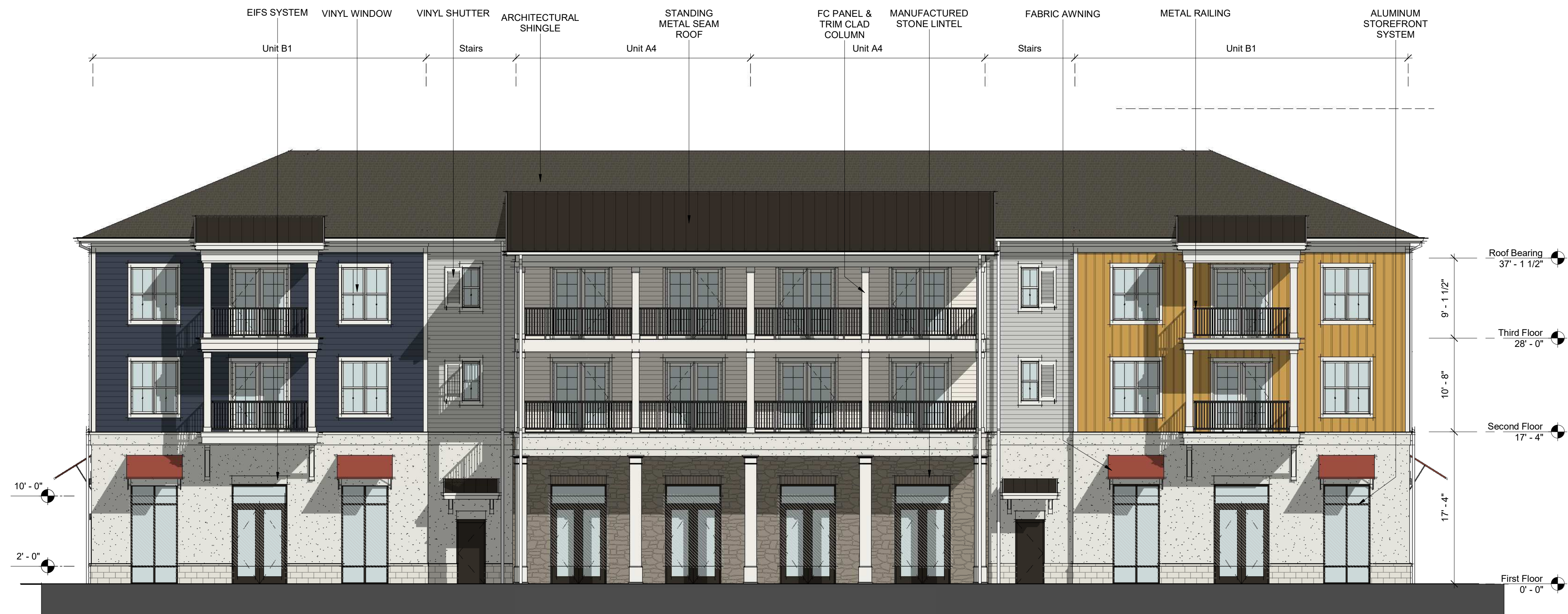
BLDG 3 - SOUTH ELEVATION 2 1/8" = 1'-0"
