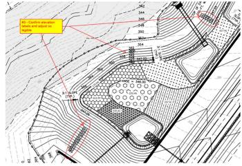
McAdams Response: The elevation labels around SCM N have been revised to align with the correct contours.
