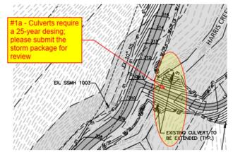
McAdams Response: The revised plans include an existing 60" culvert as the location in the snippet above. We looked at upgrading the crossing with a larger culvert, but since the 25-yr storm will overtop the greenway with or without a culvert, we are proposing to only extend the existing pipe as needed. The improvements shown should not change the current flood conditions.
