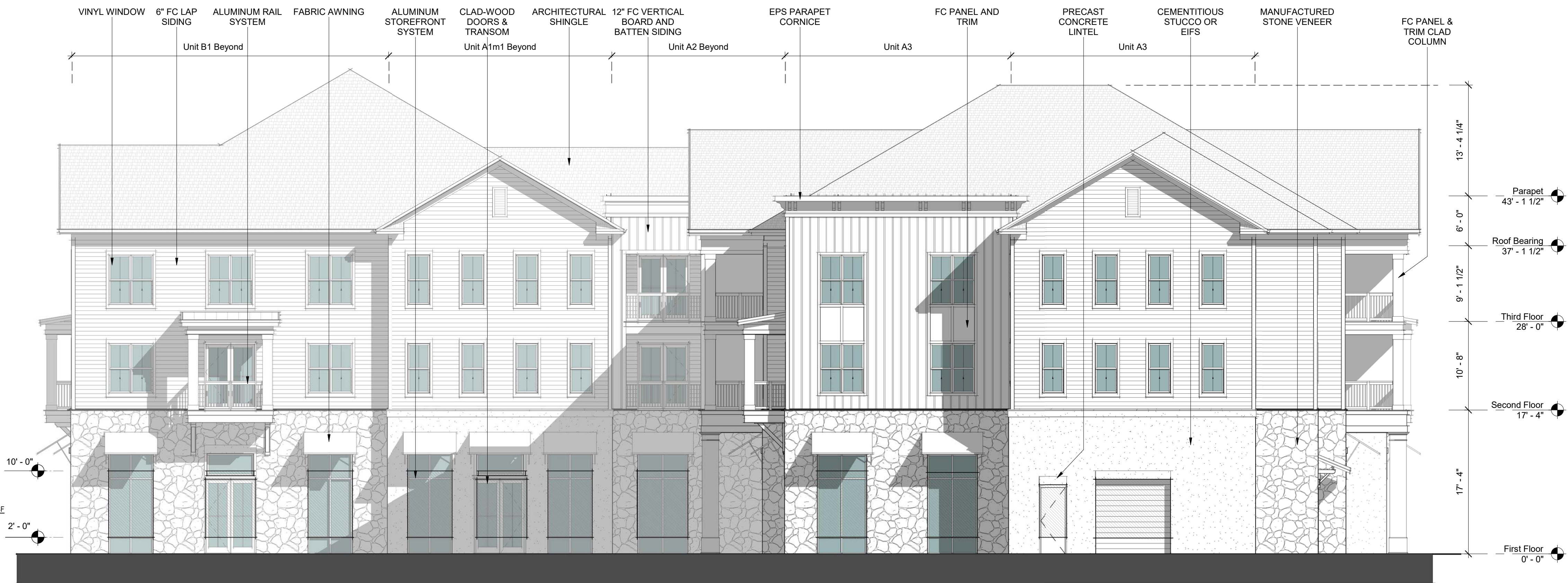
BLDG 6 - EAST ELEVATION 1 1/8" = 1'-0"
