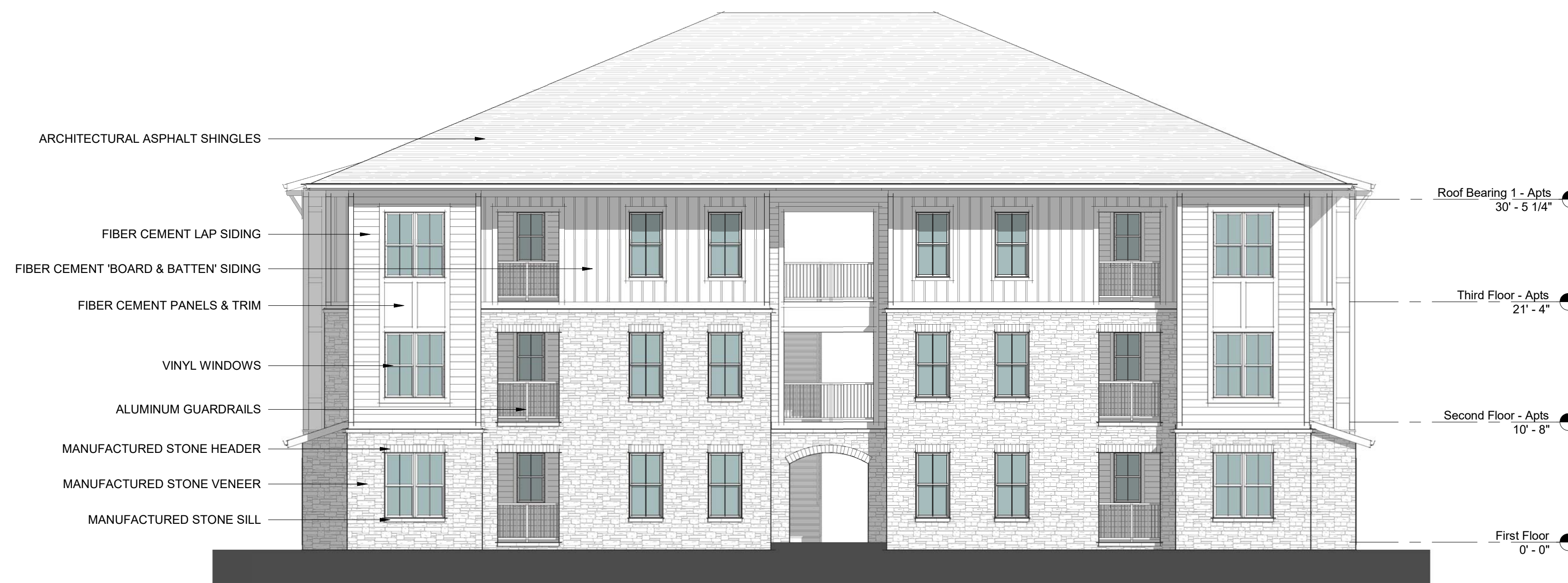
BLDG 8 - FRONT ELEVATION 1 1/8" = 1'-0"
