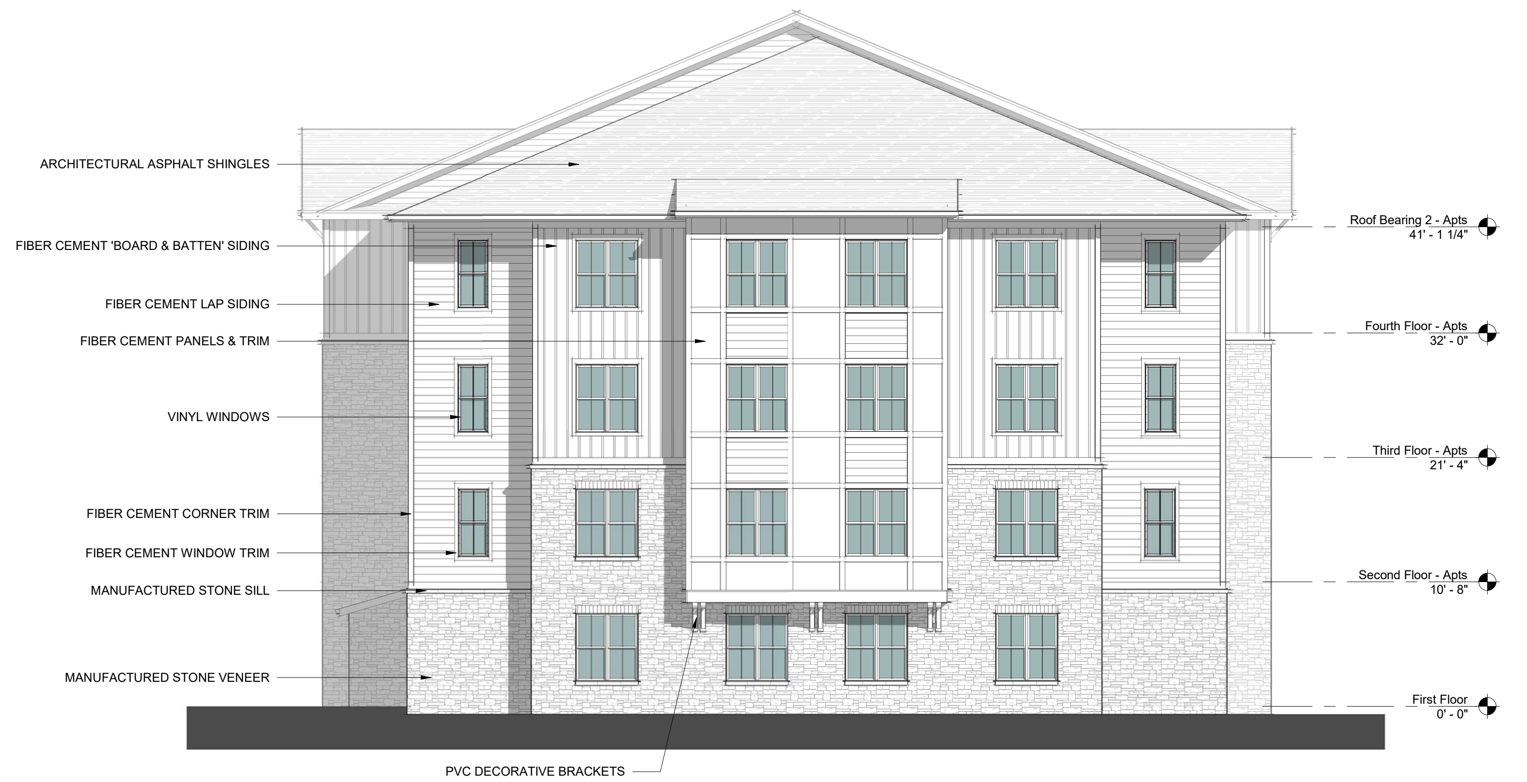
BLDG 1 & 7 - RIGHT SIDE ELEVATION 1 1/8" = 1'-0"
