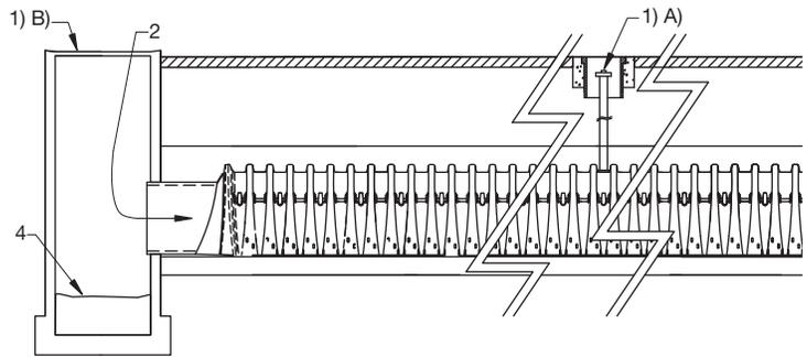
**Step 2)** Clean out Isolator Row using the JetVac process
