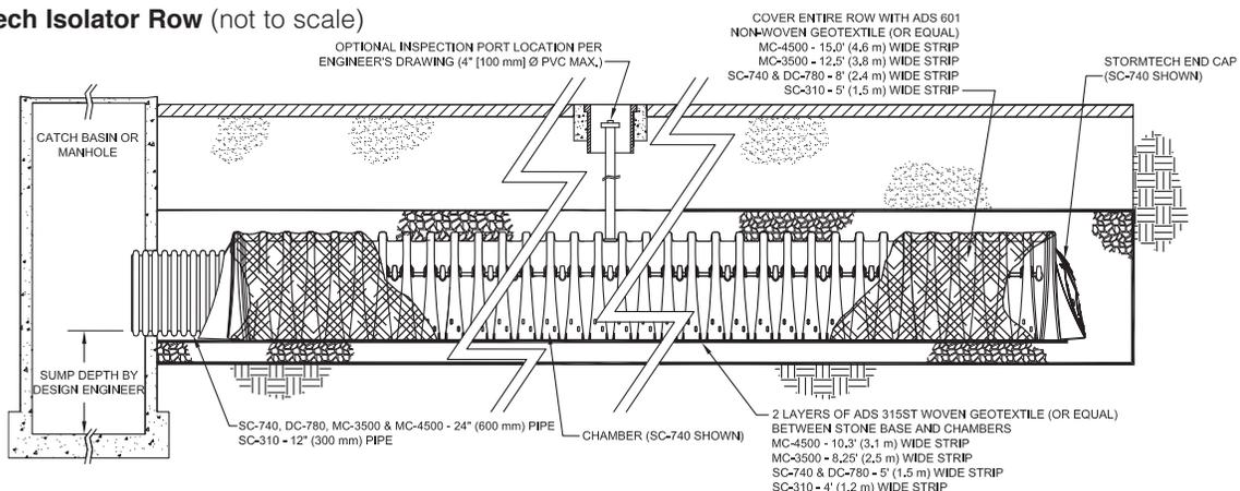
**Note:** For many applications, the non-woven geotextile over the DC-780, MC-3500 and MC-4500 Isolator Row chambers can be eliminated or substituted with the AASHTO Class 1 woven geotextile. Contact your StormTech representative for assistance.
